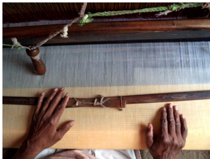
Manufacturing of Kota Doria Handloom on Pit Loom at Kaithoon
