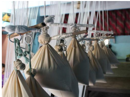
Figure : Winding of yarn using bags of sand as weighing material
